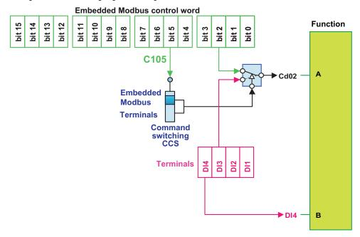
When a function is assigned to a switched bit (Cd00 to Cd15), the function can be activated via Terminals or selected communication channel according to the active command channel. To switch between Terminals and communication modules, use [Command Switching] function.
