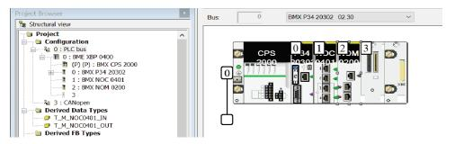
Connect a RJ45 cable between:
