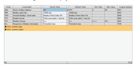
Set the [Modbus Address] to a selected address (here 14).
