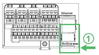
**1** Modbus RTU VP12S port is recommended to be used for communication such as with PLC.
